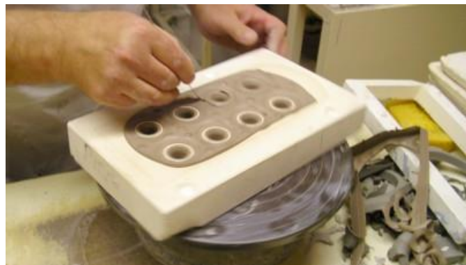
preparing to remove the thimbles from the mould
